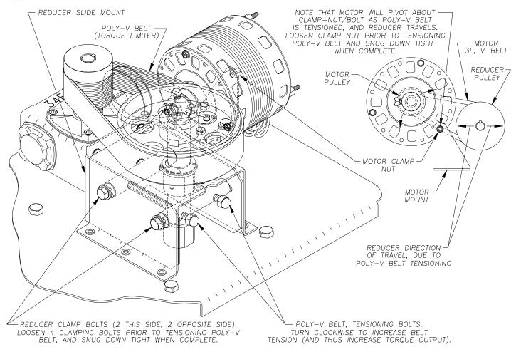
Figure 9: Torque Adjustment
